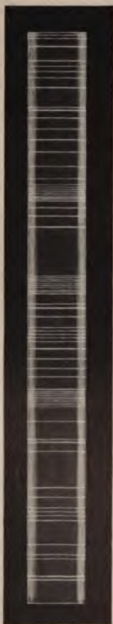
FIG. 47.—Green and blue part of the spectrum of an electric arc light.
